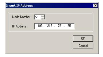
Enter the Node Number (in example 55) matching to the last octet in IP Address of computer where Omron Ethernet DAServer is running. Enter the IP Address of computer where Omron Ethernet DAServer is running (in example 195.2.103.55). Press "Ok".
